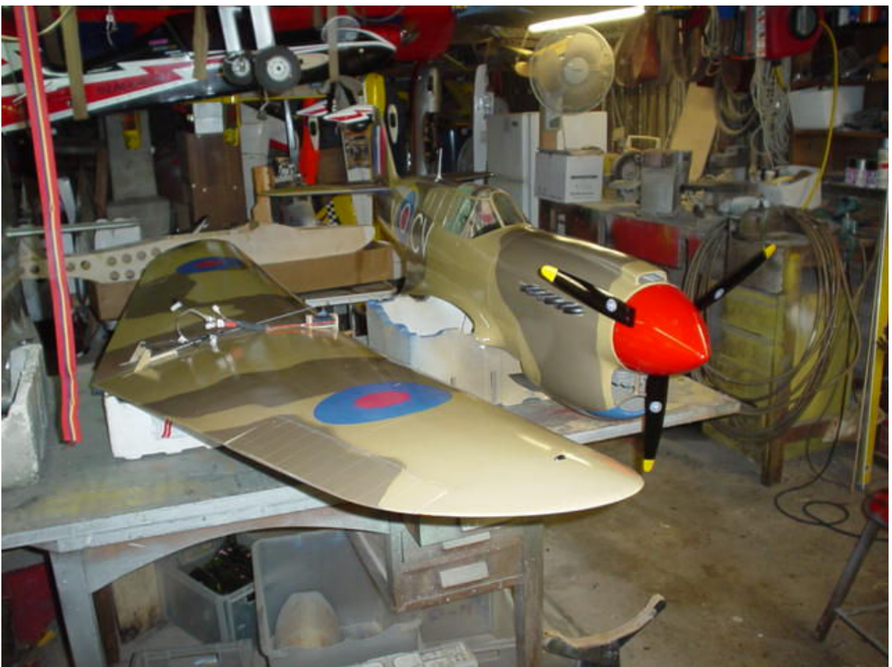
Finished spinner and prop. Prop is an old Bolly carbon 21 x 12 narrow three blader..
