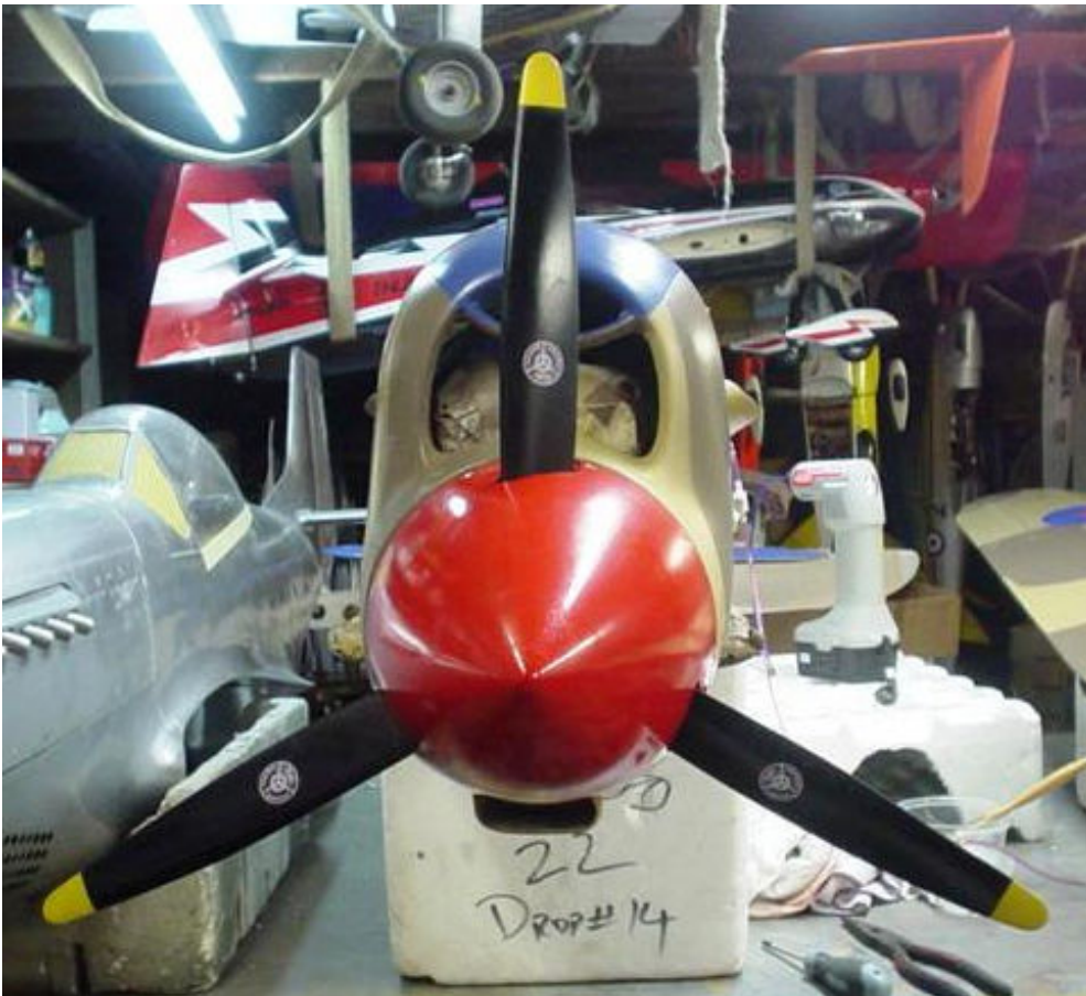
Finished spinner and prop. Prop is an old Bolly carbon 21 x 12 narrow three blader..
